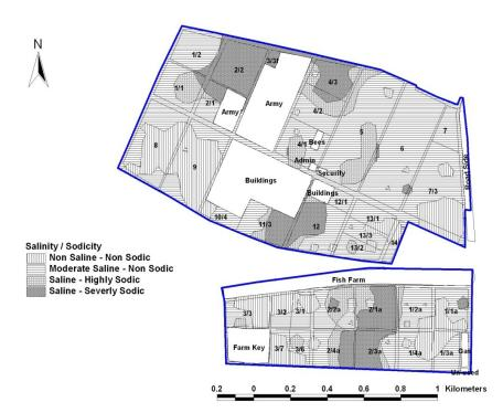
Fig. 2: Soil quality indicator map of Electrical conductivity (EC) and SAR within AbisERS
